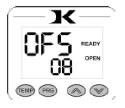
5. If the screen temperature display needs to be lowered compared to the pyrometer reading, press the DOWN arrow key.
