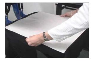
Place the Teflon sheet over the graphic, then close the heat press. After 15-20 seconds, open the press.
