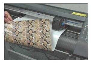
When using EnduraTEX Fashion, you will notice that the release liner is completely white. When you cut, load the colored side downwards into your cutter, allowing the white backing to be facing upwards.
