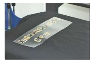
5 On your heat press, verify that your temperature is set between 300° and 340°F. If your heat press has a built in timer, set it for 15-20 seconds. Place the weeded graphic onto the cotton, polyester, or similar fabric with the release liner facing upward.
