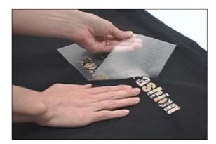
Allow the garment to cool to room temperature before removing the release liner. During this time you may remove the garment from the heat press and place in a location out of the way to allow for a second shirt pressing if desired. After the application has cooled, slowly peel the release liner away from the shirt. The garment film should remain on the fabric resulting in an image with a soft feel.
