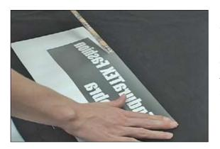
Your plotter will cut a mirror image of the original design into the garment film. When the cut-job is complete, advance the material forward and remove from the cutter using the Xacto, Olfa, or other utility or hobby knife. Using your preferred weeding tool, weed the excess material from the release liner.
