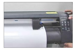
3 Next load media into the cutter. Make sure to load the media with the colored side facing down and the white side facing up. After loading the film and setting the proper cutting conditions on your plotter, perform a test cut to make sure you have proper blade depth and a weedable graphic. For cutting EnduraTEX Fashion, we suggest a standard 45° blade at about 70 grams of force. After you have performed a satisfactory test cut, send the job from your sign making software.
